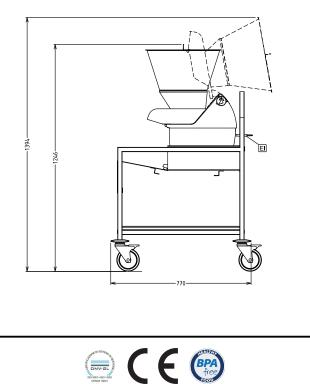
Vegetable Slicer TR210 Vegetable Slicer with Automatic Hopper on trolley - Variable Speed
