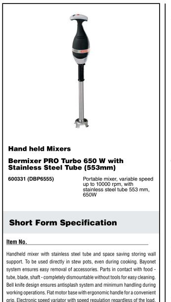
grip. Electronic speed variator with speed regulation regardless of the load. Electronic speed adjustment by pulse on + and - buttons. Maximum speed: 10000 rpm. Safety feature requires both hands to start the machine. Design for heavy duty usage: double fan system to cool down the motor. Visible and water proof (IP55) control panel to control speed levels and overload warning light. Shaft locking device avoids release during operation. Whisk accessory available as an option.
